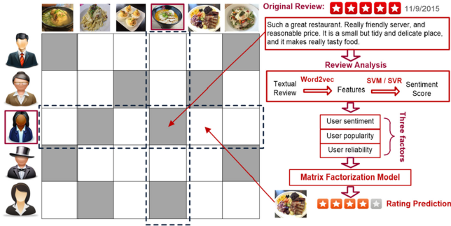
Fig. 2. An overview of our rating prediction method. Each shaded block is a review made by a user on an item. The features of these reviews are extracted by word2vec model. Then sentiment scores are calculated by SVM/SVR method. Finally, three factors, including user sentiment, user reliability, and user popularity, are fused to matrix factorization model for rating prediction.
